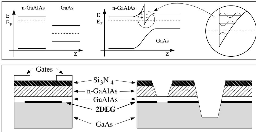
Figure 6.1: *Upper part: The mechanism leading to a 2DEG at the interface. Lower part: An undoped spacer layer between GaAs and n-GaAlAs reduces impurity scattering at the donors. The 2DEG can additionally be laterally confined by electrostatic gates (left), shallow etching (middle) or deep etching (right).*
